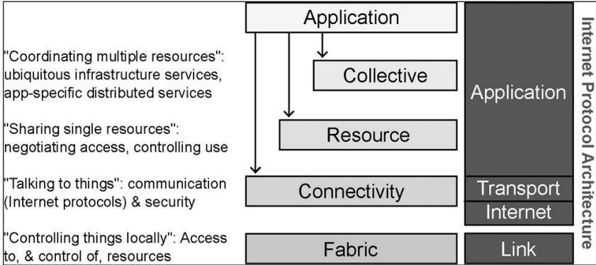
Figure 1. Grid model architecture (Abbas, 2004).
